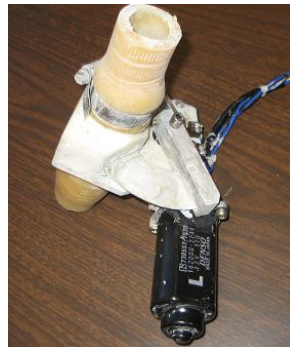
Figure 4. Mechanical Parts of the Cut-Off Valve
