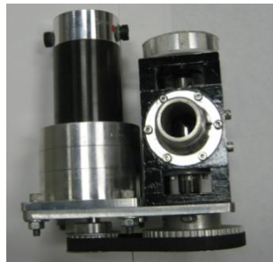
Figure 1. A new dosing pump coupled to its driving DC motor
