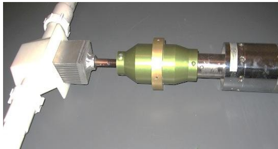
Figure 11. Vibration valve including transducer, booster and housing
