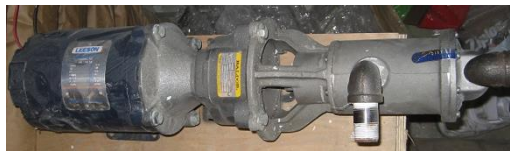
Figure 1. A progressing cavity pump driven by a large DC motor
